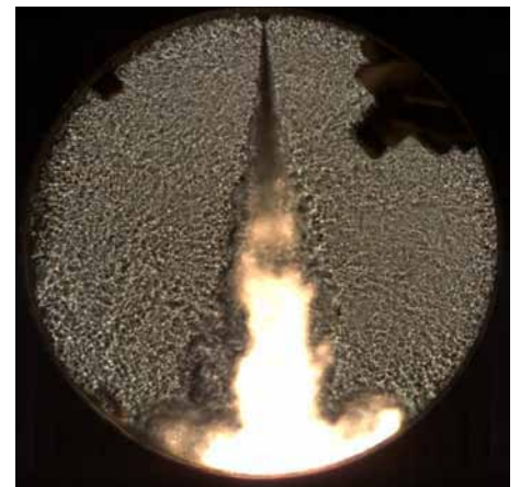
Photo Schlieren imaging of fuel injection and engine combustion 20,000fps
