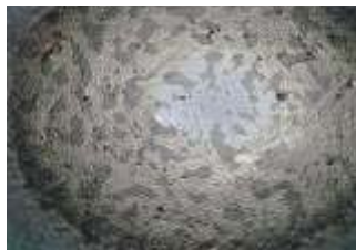
Flip-Chip焊球, 1000x
